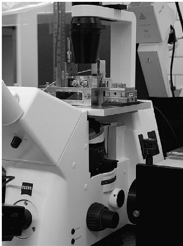
Figure 2. A photograph of a redesigned surface forces apparatus mounted on the stage of an optical microscope. Compared with the traditional design, here the crossed mica cylinders are positioned 1–2 mm away from the microscope objective, allowing the use of microscope objectives with high NA and small working distance. In addition, thermal drift has been reduced by the symmetrical mechanical placement of the working elements in this design.
