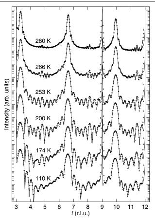
FIG. 1. Extended x-ray reflectivity of a sample with an initial thickness of 11 AL after annealing to the temperatures indicated. Curves are fits that reveal the relative coverage of different film thicknesses present on the sample surface. The sharp peaks at l = 3, 9, and 12 are Bragg peaks from the Si(111) substrate, and the broad peaks at  $l \approx 3.3, 6.6, \text{ and } 9.9$  are Bragg peaks from the Pb(111) overlayers.
